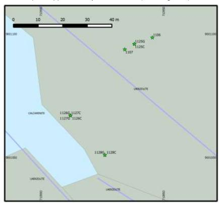
Figure 1: Simplified geology map showing sample locations. Samples 1106 and 1128 are approximately 50 metres apart.
